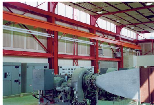
The solution involved covering about 50% of the ceiling (6,602 sq. ft.) and about 10% of the walls (2,069 sq. ft.) with the EFPs. For the ceiling treatment, three-quarters of the panels are 30 in. by 10 ft.; the remainder, 30 in. by 8 ft. On the walls, Eckel installed a mix of panels measuring 48 in. by 8 ft. and 24 in. by 6 ft. (All of these are standard EFP sizes.)
